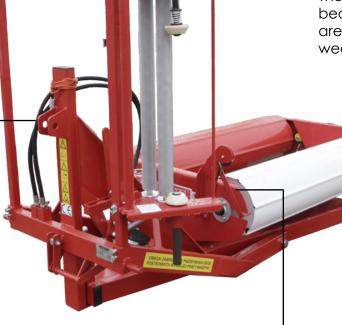
The ribs on the bale wrapper drums improve their durability and prevent sliding of the bale.
